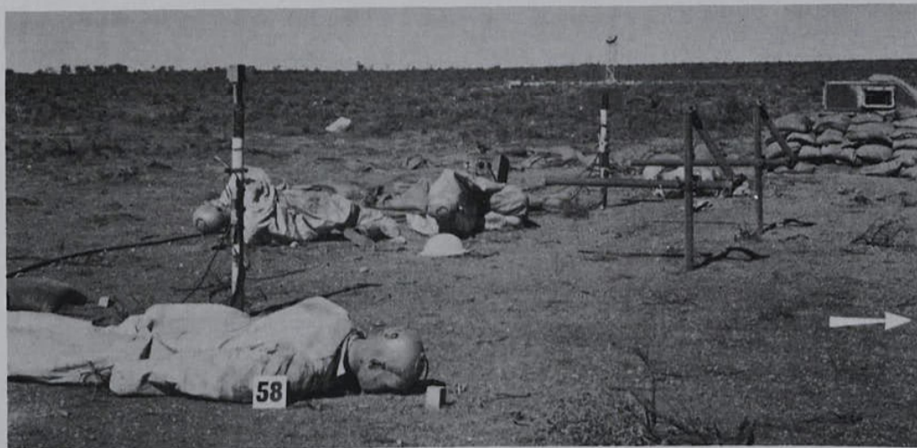
FIGURE 9. ROUND 2. DUMMIES AT 2200 ft. NOTE WHITE NAILS IN FRONT OF PRONE FACING DUMMY USED AS A REFERENCE MARK
